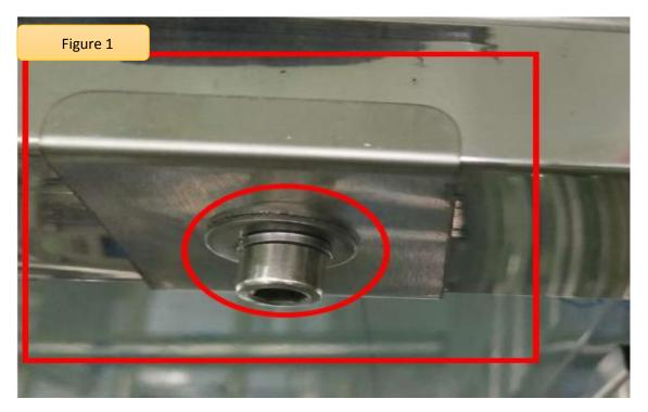
The first step;Use M8\*40 hexagon socket screw (9) to add flat cushion spring washer and baffle plate (6) to install large guardrail and top box on both sides (Figure 1).
