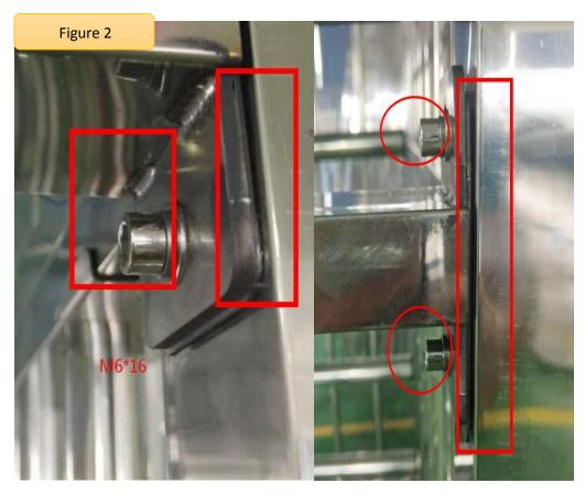
Step 2: Use M6\*16 screws (8) and baffle plates (5) and (7) to install the guardrail with card brush panel to the large guardrail (install one side first, install the other side after the middle rotary rod is installed) (Figure 2)
