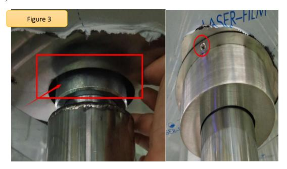
Step 3: Pre-place the sleeve (11) and upper cover (12) on the rotating rod, and then but the rotating rod with the clamping slot of the movement. Then use three M4 screws (3) to install the upper cover on the top box, and install the bottom of the rotating rod on the bearing base (10) (Figure
