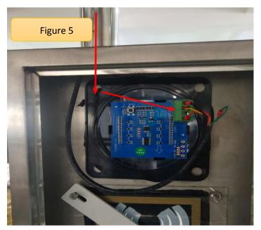
Step 5: Connect the indicator cable through the top box and the inner wall of the guardrail pipe to the installation box of the guide reading head, and connect the terminal (Figure 5)
